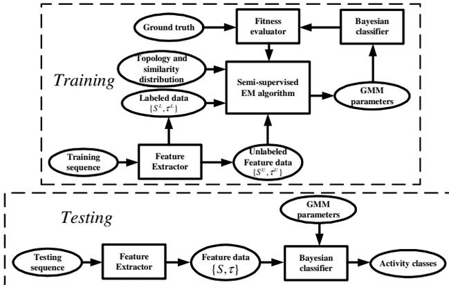
**Figure 1.** The dataflow diagram of the proposed SS EM-based human activity classification method.
