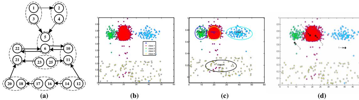
**Figure 2.** (a) The topology of the simulated camera network with 25 nodes and 13 directed links; (b) The simulated feature points in the activity behavior space; (c) the estimated Gaussian Mixture Model by the semi-supervised EM algorithm, which captures the property of the simulated data; and (d) the estimated class centers by using the unsupervised K-means clustering, which severely deviate from the true class centers.
