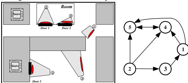
**Figure 3.** (Left) Experiment setup of the camera network showing their locations, FOVs (shade areas), and entry/exit points of the cameras (red ellipses), and (right) the topology of the real-life camera network.
